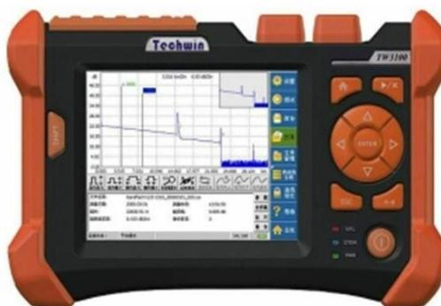
Gambar 9 - OTDR : Techwin TW3100 ([www.diytrade.com](http://www.diytrade.com))
