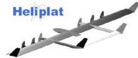
HELINET project Heliplat (Artist's Impression) (Politecnico di Torino) Wingspan: 70m Payload: 100kgr
