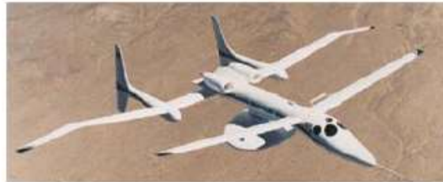
Angel Technologies HALO (Proteus 9) Manned aircraft for the delivery of communication services
